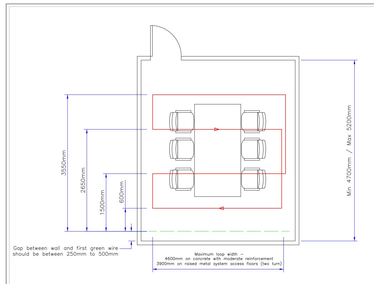
This design is intended for rooms with a Y dimension between 4.7m and 5.2m, the gap at the top and bottom of each array should be increased or descreased accordingly to keep the loop dimensions exactly as shown. In the X axis the design can be extended to fill the room up to the limits provided on page 1.
