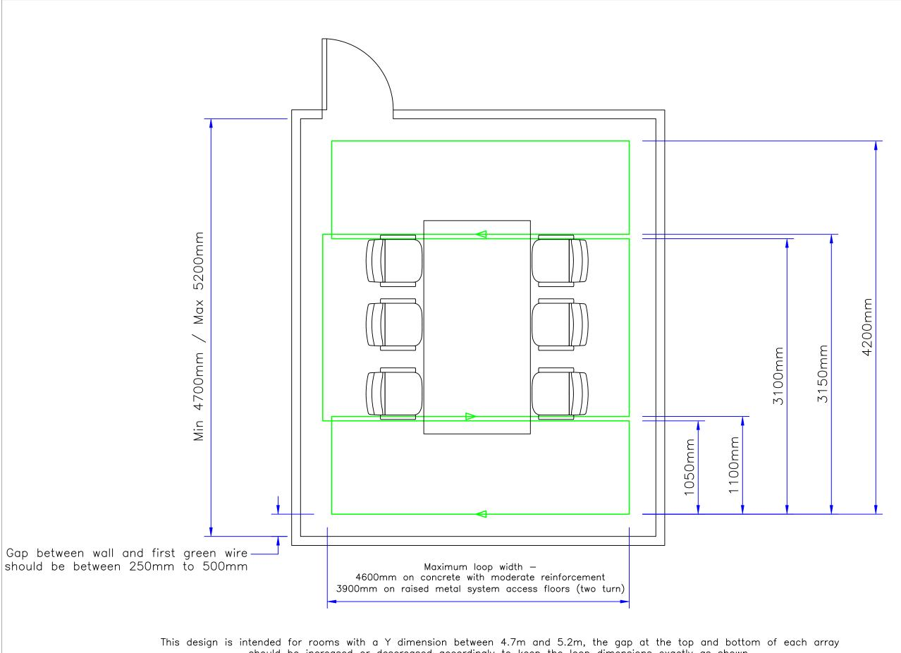
should be increased or descreased accordingly to keep the loop dimensions exactly as shown.
